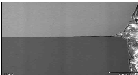
FIGURA 38-Implante 3i com abutment gold UCLA - amostra 1. Aumento 500x
